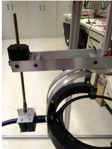
Figure 9: Real picture of helmet with rotational movement part
